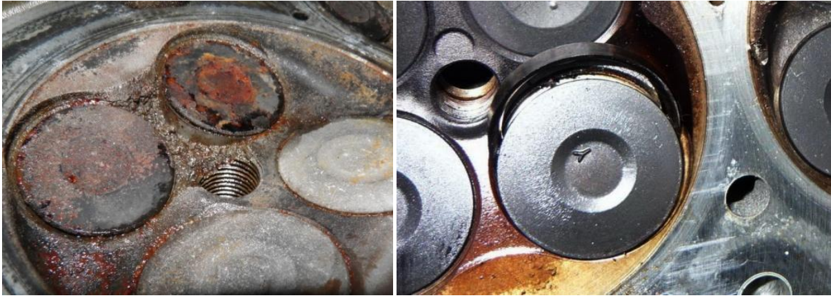
Fig. 4. A combustion chamber with traces of the wall melting between the exhaust valve seats (left) and a case of seats falling out due to overheating when the engine is running in place (right)
